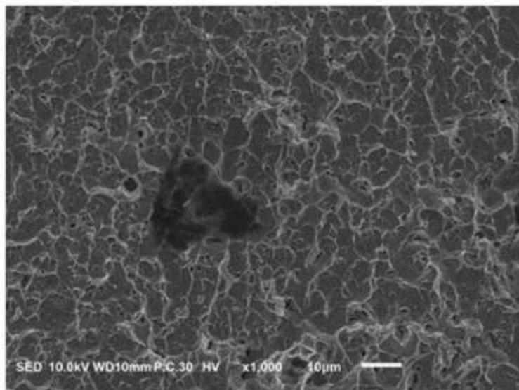
**Figure 1. The SEM Surface Of PTU In Static Cycles. There Is No Striation On The Entire Image.**
