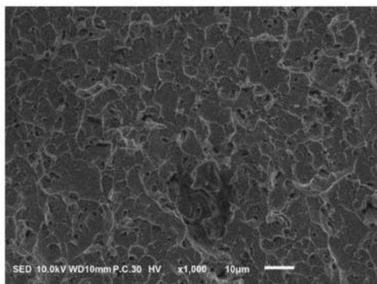
**Figure 2. The SEM Surface Of PTU In Dynamic Cycles. There Is No Striation On The Entire Image.**
