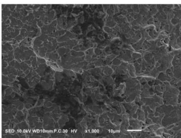
**Figure 3. The SEM Surface Of PTN In Dynamic Cycles. There Is No Striation On The Entire Image.**
